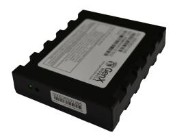
The best place to mount the unit is in an area with little to now metal blocking above the unit. Most areas in the dash of the vehicle will work just fine. AVOID areas such as underneath the radio as this would completely cover the unit in metal.
