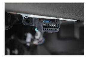
Above image displays the OBDII port location in the lower driver side dash of the vehicle. The J-Bus port is generally located in the same area in heavy trucks.
