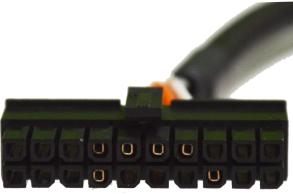
Above image displays the power harness plug which connects to the FieldLogix GPS Device
