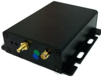
Find a secure location underneath the dashboard to mount the GPS device. Do not mount device under the hood of the vehicle or in the engine compartment. The heat from any of these locations may cause product failure.
