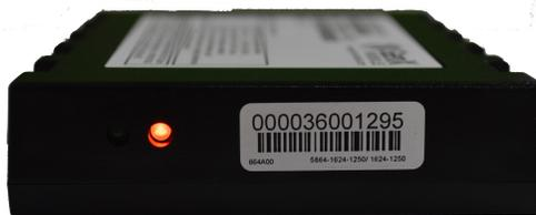
The RED LED flashes 2-digit codes. Roughly speaking the first digit tells you what general area is having a problem (hardware, modem, GPS, end-end service). The second digit gives specific error information. Since there can be more than one error condition the unit rotates through the error codes (for example if GPS is tracking no satellites and the modem is not registered).
