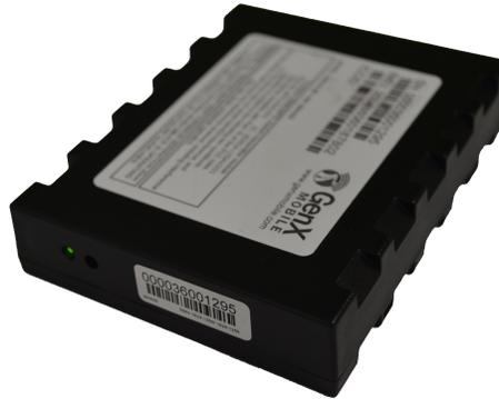
The best place to mount the unit is in an area with little to now metal blocking above the unit. Most areas in the dash of the vehicle will work just fine. AVOID areas such as underneath the radio as this would completely cover the unit in metal.
