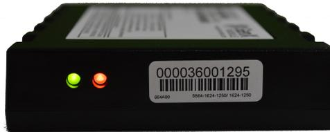
The Diagnostic LEDs will indicate if the unit is having issues with communication, GPS fixing and more. It is also recommended that the data server be checked to confirm that report data is arriving.
