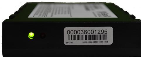
The unit will power up as the vehicle's ignition is turned on. The Green LED will show solid for approximately 30 seconds (there may be some brief flickers initially while the processor initializes). At no other time should the green LED remain on solid for such a long period. After 30 seconds the green LED will start to flash at the following rates:
